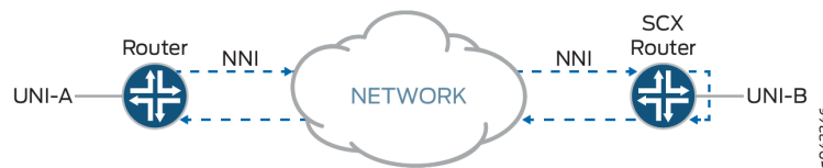
Figure 72: Testing End-to-End Service in Ethernet Loopback Mode
